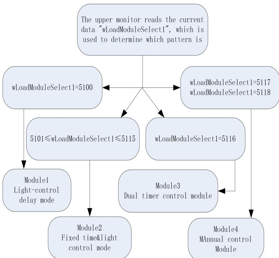
④ Light-control delay mode (5100): starting voltage (can be set), closed voltage (can be set), action time delay (can be set);
