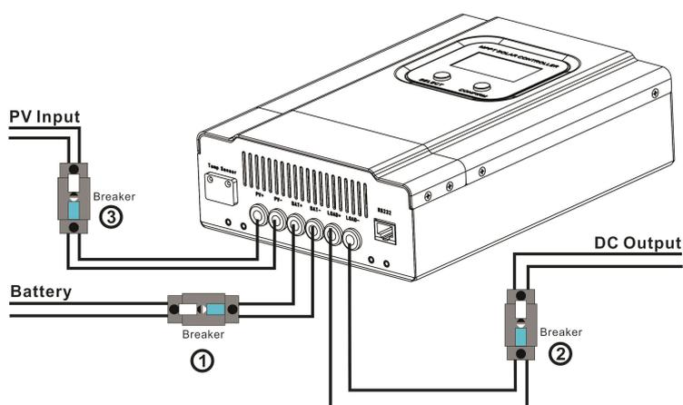
**Make sure that the controller is installed and connected as above**
